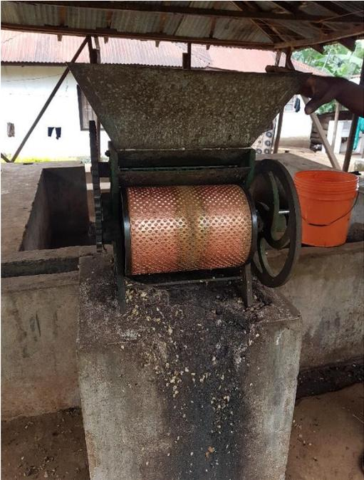
**Pictures 1 and 2:** the wet mill used by one of the base cooperatives in the Kilimanjaro region. The mill itself is powered by hand.
